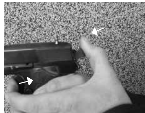
Fig.3> Pistol M88 blocking when the hammer is cocked
