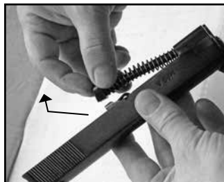
Fig. 10> Taking out the recoil mechanism (recoil spring with guide)
