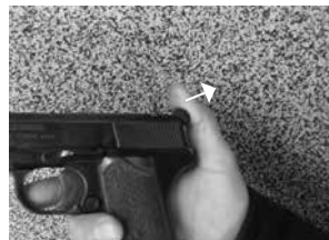
Fig.4> Pistol M88 blocking when the hammer is down
