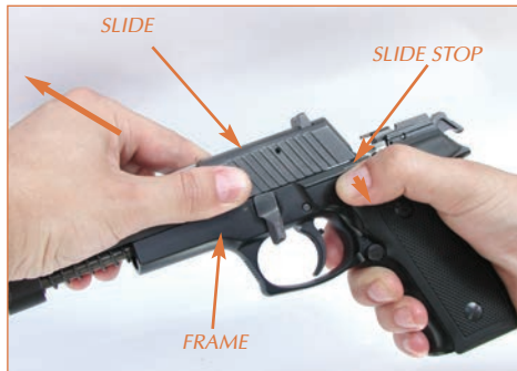
Fig. 11 SEPARATING SLIDE FROM THE FRAME
