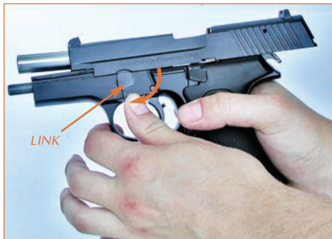
Fig. 10 SWIVELING BARREL LINK
