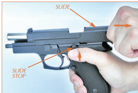
Fig. 9 PULLING SLIDE BACK IN THE REAR POSITION
